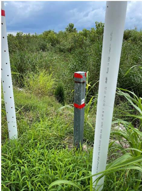
Photograph No. 9 Pond 003 Monitoring well on upstream slope of eastern embankment
