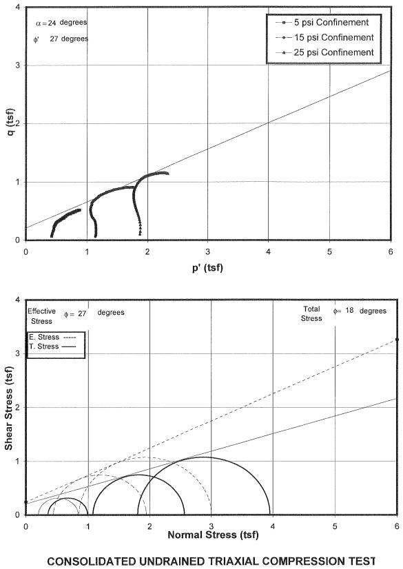
ASTM D 4767 Project No.: J011309.02 Boring: B-2 Sample: ST4 - Depth: 7
