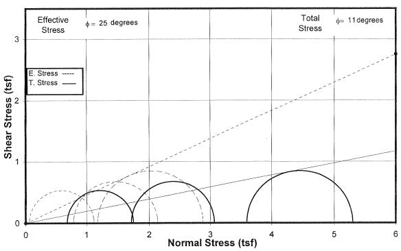
ASTM D 4767 Project No.: J011309.01 Boring: C-2
