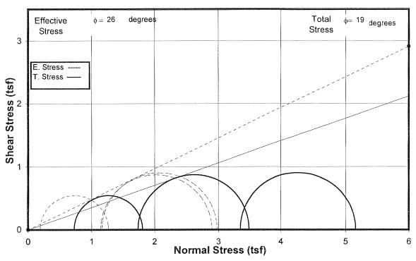
ASTM D 4767 Project No.: J011309.01 Boring: C-1
