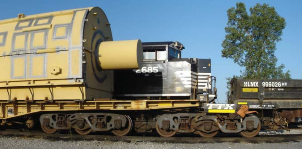
When moving the Chouteau 2 components from Arizona, including this generator, each rail car was monitored electronically and by personnel traveling with the train to ensure safe delivery.
