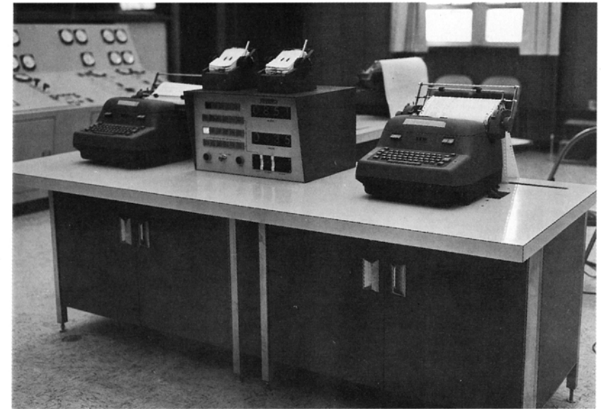
Crude by today's standards, these computers in Thomas Hill Unit 1's control room help to operate the plant in 1966. Two IBM typewriters connect to the computer unit in the middle which processes information from points throughout the plant. The computer transmits alarms to the typewriters which print a list for control room operators.
