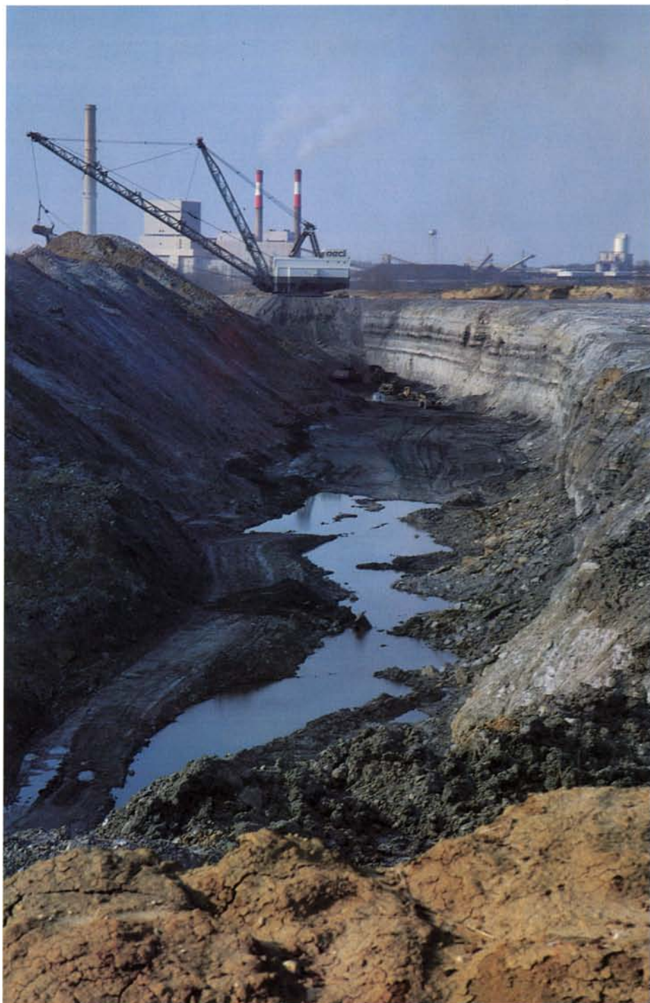
One of Associated's three draglines uncovers coal at the end of a long pit near the power plant at the Thomas Hill Energy Center in the mid-1980s.
