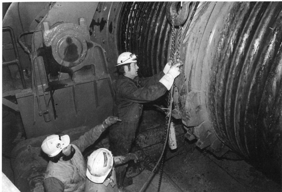
Mining Division employees Joe Lewis, right, and David Cheever, left, install new steel ropes on a dragline drum.
